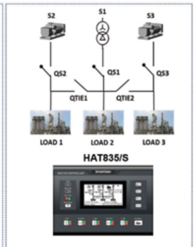
Tri-supply control module with 2 bus ties
