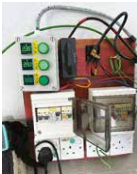
Figure 9. Field test set with functional and faulty RCDs.
