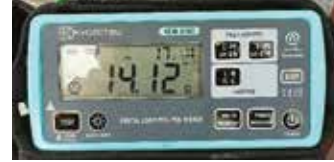
(c) Earth loop impedance test -- Earthing rods without connection to foundation steel re-inforcing bars
