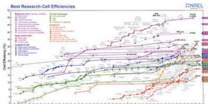
Figure 2: Solar PV Efficiency Trends Best Research-Cell Efficiency Chart
