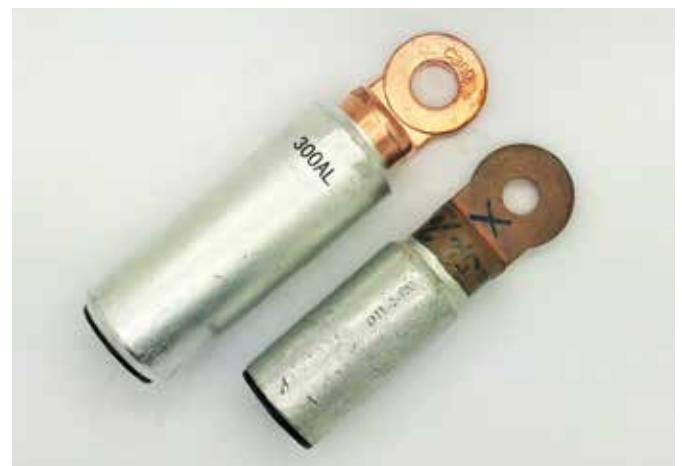
Comparison between a Standard-compliant and Sub-standard 300mm² Bi-metal Lug
