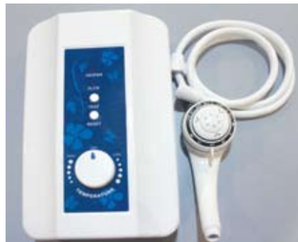
Instantaneous water heater – Chrome type or metalised plastic shower head and metallic hose must be replaced with rubber/non conducting type.
