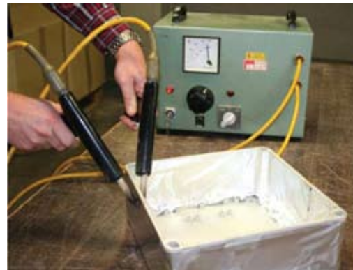
The HENSEL KV-, ENYSTAR- and Mi-distributors have passed the insulation test in the Hensel quality assurance with 4665 V. Therefore these distributors are suitable for the operation of U_{oc} = 1000 \text{ V} .
