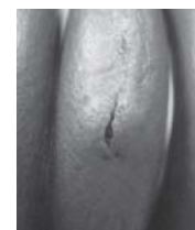
Picture 3 - A punctured heating element protection sheath.
