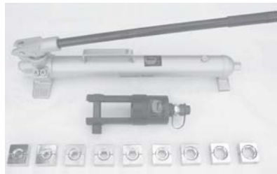
CP-400 Hydraulic Crimping Tool Dies: 50mm 2 to 400mm 2
