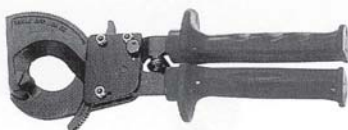
Model: LK-300B Ratcheting Cable up to 325mm 2
