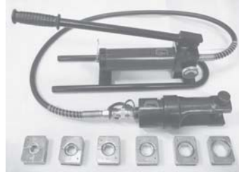
CP-630 Hydraulic Crimping Tool Dies: 185mm 2 to 630mm 2
