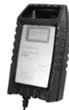
CHK Gridsense PM40 Power Quality Analyser
